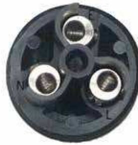
Figure 5: Wire Connections Brown wire to terminal L Blue wire to terminal N Green/Yellow wire to terminal E
