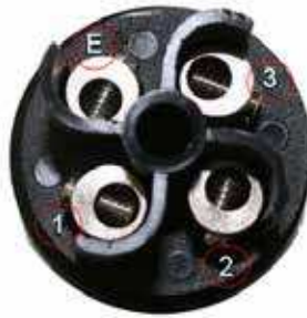
Figure 6: Wire Connections Brown wire to terminal 1 Black wire to terminal 2 Grey wire to terminal 3 Green/Yellow wire to terminal E
